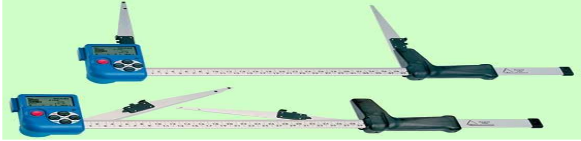
Figure 18. Computer caliper gauge Haglof Digitech Professional, produced in Sweden
